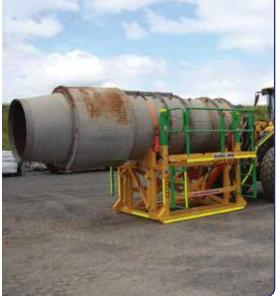
The QMW dynamic fan and silencer service platform is designed to provide a stable, robust and safe platform for underground applications, in compliance with AS1418.10, EN280:2001 and MEWP standards.
