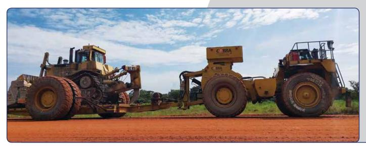
This 120 ton Tilting Low Loader is rear-loading, designed specifically for rapid load/unload and one person operation, which facilitates short distance repositioning of tracked equipment.
