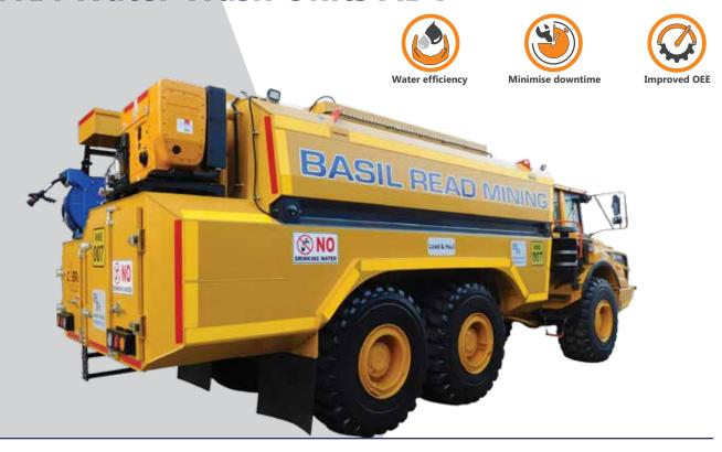
To rapidly and effectively prepare large machines for maintenance, Cobra has designed dedicated wash units to simultaneously clean booms, tracks, platforms and specific work areas by using multiple high pressure and high volume washing outlets.
