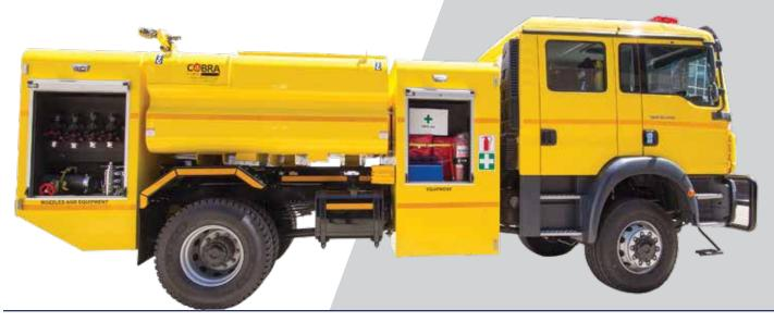
European style medium-major fire and rescue pumper, mounted on a commercial 4x2 or 4x4 chassis, single or crew cab, specifically designed for the mining environment.
