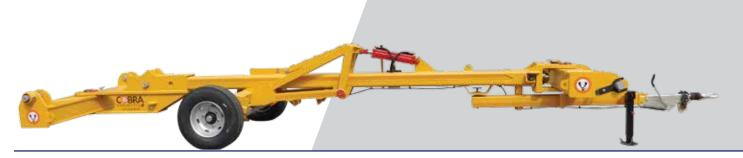
The rigid tow links are for towing broken down dump trucks in a safe manner.
