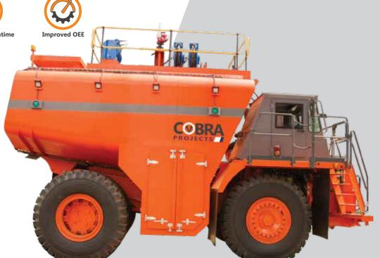
To rapidly and effectively prepare large machines for maintenance, Cobra has designed dedicated wash units to simultaneously clean booms, tracks, platforms, and specific work areas by using multiple high pressure and high volume washing outlets.
