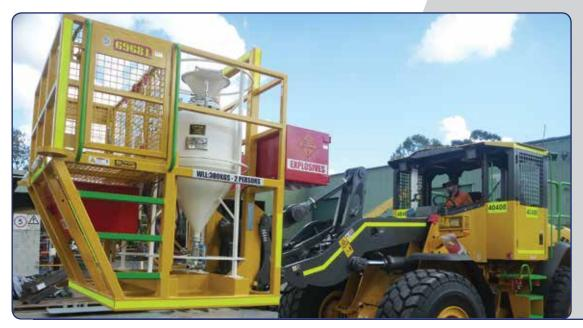
The ANFO underground work platform is designed to provide a stable, robust and safe platform for underground applications. This equipment comprises two pressure pots used for the underground loading of ANFO, and is designed in compliance with AS1418:10 standards.
