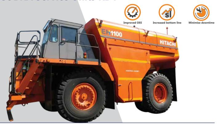
To minimise service time of very large machinery, we offer high flow rates of multi-products, from diesel to grease, on large RDT chassis.
