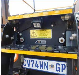
The ADE all electric access system is a step ladder access design that can be fitted to most mining, earthmoving and rail equipment. This access system is designed in compliance with AS1657-2013 & AS3868-1991 standards. Requiring no hydraulic power pack for operation means a very competitively priced access system solution. This system can be fitted to mobile equipment requiring a powered folding step ladder-type access solution.
