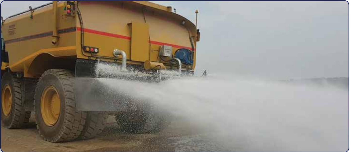
These units offer up to 16 metres of road spray coverage and can be equipped with machine washing and/or firefighting capabilities.
