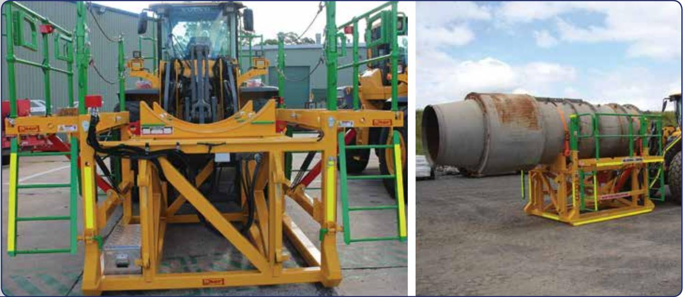
The QMW dynamic fan and silencer service platform is designed to provide a stable, robust and safe platform for underground applications, in compliance with AS1418.10, EN280:2001 and MEWP standards.
