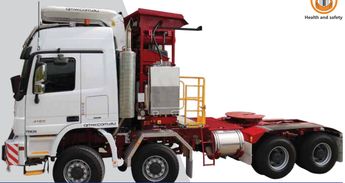
To protect drivers and passengers, Cobra manufactures, under license, the QMW range of ROPS (ISO 3471 certified) and FOPS (ISO 3449 certified) for HDV equipment. The range has structural optimisation through the use of finite element analysis (FEA) and certified destructive testing, combined with contemporary styling techniques. Q-ROPS provide a lightweight, cost effective and value adding solution for full mine compliance on any make and model of truck.
