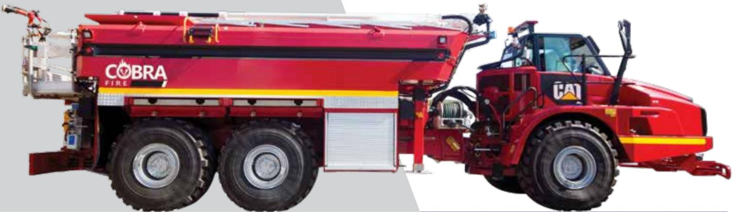
Cobra offers a range of firefighting units from drop-in units suited to Land Cruisers through to units that mount on ADT's. Units can be equipped with CAFS and/or AFFF.
