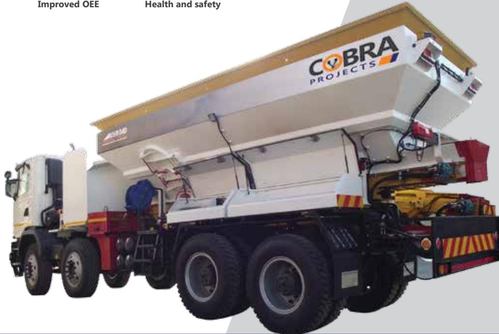
This unit offers the ability to complete a bench of 200-300 holes in one shift with one operator, with a pre-set amount of stemming placed into each hole. No more relocation of stockpiles as the unit can run a few kilometres to the stock yard and there is also no wastage of aggregate when filling the holes.
