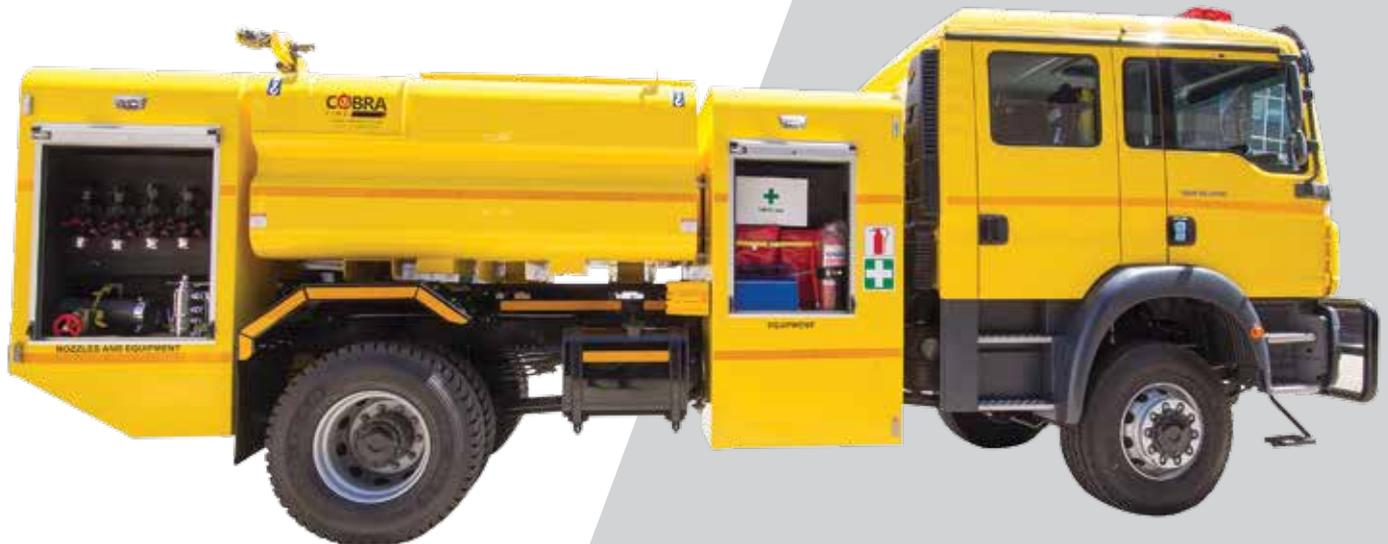
European style medium-major fire and rescue pumper, mounted on a commercial 4x2 or 4x4 chassis, single or crew cab, specifically designed for the mining environment.
