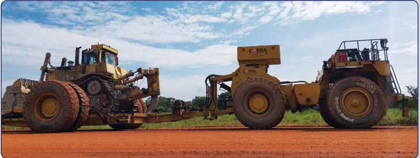
This 120 ton Tilting Low Loader is rear-loading, designed specifically for rapid load/unload and one person operation, which facilitates short distance repositioning of tracked equipment.
