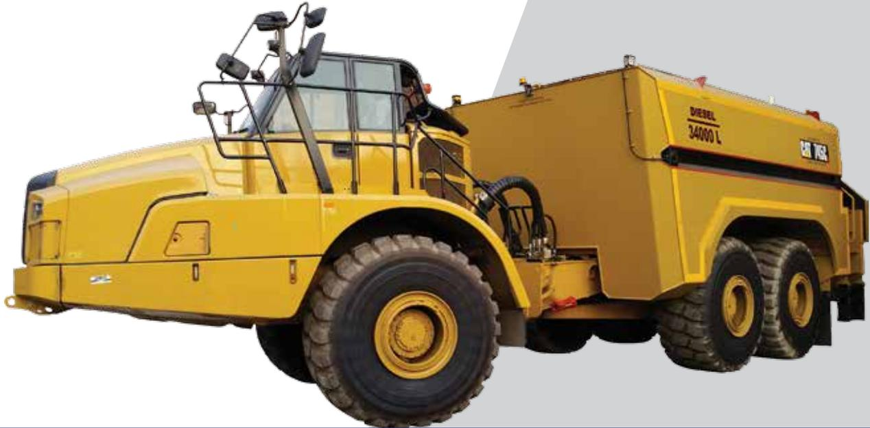
To rapidly replenish the daily diesel consumed, our bowzers offer high and low volume dispensing from the same pump and filter arrangements.
