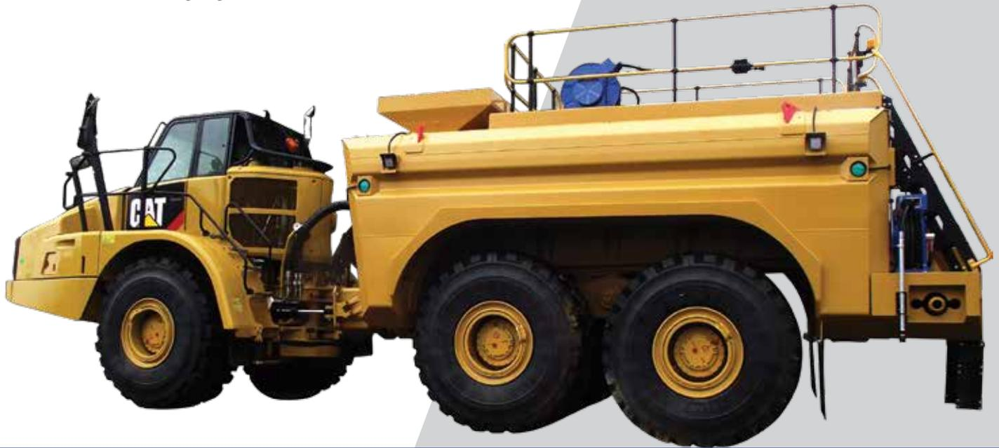
These units offer up to 16 metres of road spray coverage and can be equipped with machine washing and/or firefighting capabilities.
