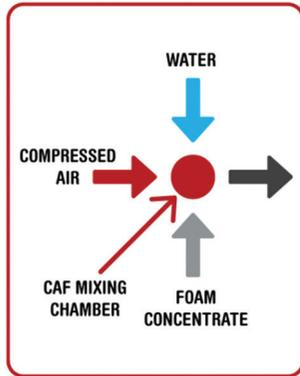
All CAFS work off the principle of combining a foam solution with compressed air. A mixing chamber is required to achieve the necessary bubble structure which plays a pivotal role in the effectiveness of managing fires. Foam may be introduced either at or before the mixing chamber.
