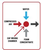
All CAFS work off the principle of combining a foam solution with compressed air. A mixing chamber is required to achieve the necessary bubble structure which plays a pivotal role in the effectiveness of managing fires. Foam may be introduced either at or before the mixing chamber.
